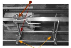
4) Cradle rods slide through holes in adjuster bar (left) and cradle forks (right); anchor in place with set screws DO NOT OVER TIGHTEN SCREWS OR BOLTS!
