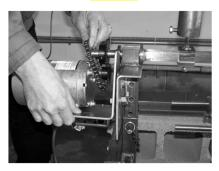
5) Lift swivel plate up to place or remove chain from sprockets;
